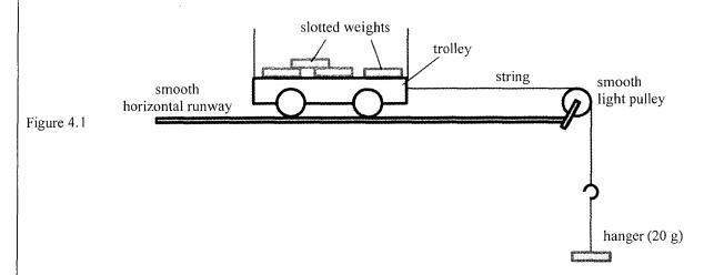
The experiment is repeated by transferring the slotted weights one by one from the trolley to the hanger so as to increase the mass hanging, m.
