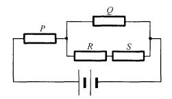
If the power dissipated by R is 1 W, find the total power output of the battery.
