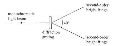
When a monochromatic light beam is incident normally on a diffraction grating with 300 lines per mm, a pattern of bright fringes is formed. The angle between the two second-order bright fringes is 40°. Find the frequency of the light.
