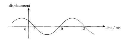
The displacement-time graph of a particle on a travelling wave is as shown. Find the frequency of the wave.
