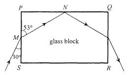
The figure shows the cross-section of a rectangular glass block PQRS. A light ray is incident from air at M on face PS and the refracted ray strikes face PQ at N. Find the critical angle for the glass-air interface.
