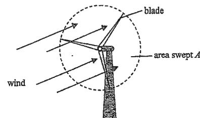
(a) By considering the amount of air passing through the wind turbine in one second and assuming that about 35% of its kinetic energy is converted to the mechanical energy of the turbine, show that the wind turbine delivers a power of  $k \rho A v^3$  and find the values of the constants  $k$  and  $n$ . (5 marks)
