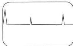
Figure 3 shows the CRO display of the test result on a certain day. The engineer points out that there may be a small crack in the wall of the pipe. Explain how the engineer arrives at such a conclusion. (2 marks)
