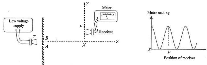
The figure above shows a set-up to investigate the interference of microwaves. Microwaves emitted from a transmitter  $T$  pass through two narrow slits  $A$  and  $B$ , which are equidistant from  $T$ . The receiver is then connected to a meter, which indicates the intensity of microwaves received.
