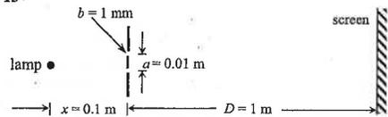
A student prepares a double-slit interference experiment as shown.  $a$  is the slit separation and  $b$  is the slit width. However, no interference fringe can be observed on the screen. Which of the following improvements should be taken ?
