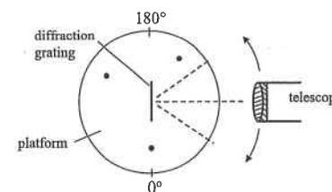
To observe the light spectrum of the sodium lamp, a student places a diffraction grating on a platform such that the incident light falls normally on the grating. There is a protractor scale on the platform from  $0^\circ$  to  $180^\circ$ . The sodium lamp produces a yellow light of a certain wavelength. The student uses the second-order images and records the angular position readings of the yellow line on each side of the central line as follows :
