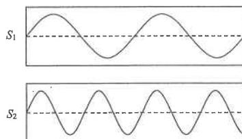
Two tuning forks  $F_1$  and  $F_2$  are hit respectively to give sound notes. Their waveforms are displayed on a CRO connected to a microphone. The traces  $S_1$  and  $S_2$  observed on the screen of the CRO are given by  $F_1$  and  $F_2$  respectively. The time base of the CRO remains the same in each case. Which of the following statements is/are correct ?
