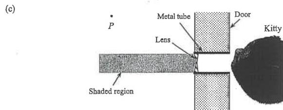
The Figure above shows the top-view of the peephole. The metal tube will only allow Kitty to see those images formed in the shaded region. Now a visitor stands at a point  $P$  and Kitty cannot see him through the peephole.
