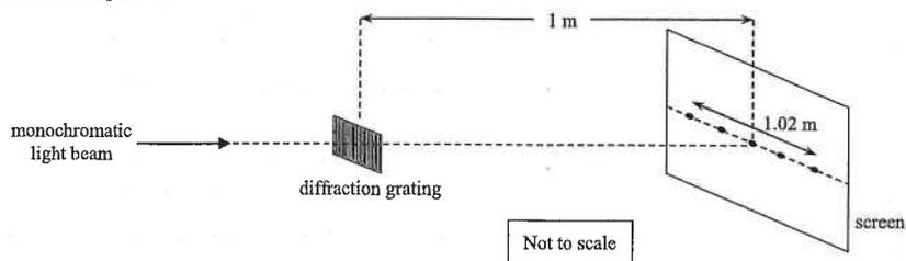
Monochromatic light of wavelength 570 nm from a laser is directed normally onto a diffraction grating as shown. A screen is placed at a distance 1 m behind the grating. The central part of the resulting diffraction pattern is shown in the figure. The separation between the second-order bright spots on both sides of the pattern is 1.02 m.
