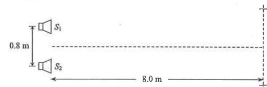
Two loudspeakers  $S_1$  and  $S_2$  are connected to a signal generator to give out sound waves that are in phase. The separation between  $S_1$  and  $S_2$  is 0.8 m. A student moves a microphone along a line  $PP'$  8.0 m away from the loudspeakers and parallel to  $S_1S_2$ . Loud sound is detected consecutively at  $P$ ,  $O$  and  $P'$ . If  $PP'$  equals 2.0 m, estimate the wavelength of the sound produced by the loudspeakers.
