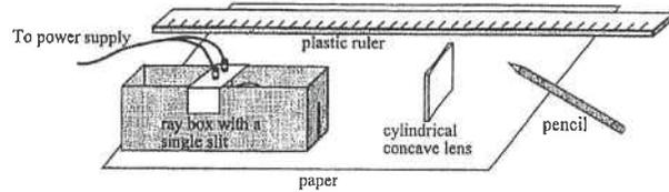
Describe how you would use the above apparatus to find the focal length of the lens and state ONE possible source of error in the experiment. (5 marks)
