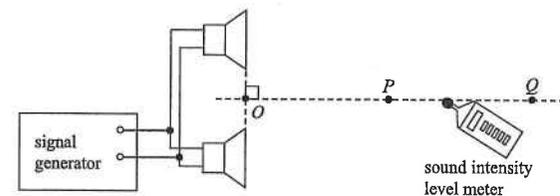
Two identical loudspeakers are connected in parallel to a signal generator,  $O$  is the midpoint between the loudspeakers. When a sound intensity level meter is moved from  $P$  to  $Q$ , the graph below shows the variation of the sound intensity level received with position.
