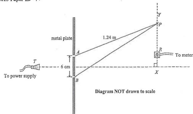
The Figure above shows a set-up for the study of interference of microwaves. Microwaves of wavelength 2 cm emitted from a transmitter  $T$  pass through two slits  $A$  and  $B$  formed by metal plates. The slits are separated by 6 cm as shown. A probe  $R$  connecting to a meter is moved from  $X$  to  $Y$  to detect the intensity of microwaves received. Transmitter  $T$  and point  $X$  are equidistant from  $A$  and  $B$ .
