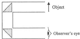
A student uses two triangular prisms to construct a periscope as shown above. Which of the following shows the image of the object as seen by the observer?
