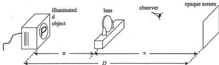
Kitty uses the set-up in the above Figure to study the image formation of a lens. The lens is placed at a distance  $u$  from an illuminated object (letter 'P'). An opaque screen is placed at a distance  $D$  from the object so as to capture the image.
