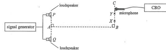
The above Figure shows two identical loudspeakers P and Q connected to a signal generator. Position A is the mid-point of PQ. A microphone connected to a CRO is moved along BC. The amplitude of the CRO trace increases as the loudness of the sound detected increases. The Figure below shows how the amplitude of the CRO trace varies with the position of the microphone.
