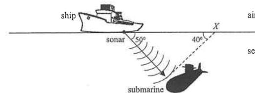
A ship equipped with a sonar system is used to detect objects in the sea. Ultrasound of frequency 25 kHz are sent towards the seabed. The ultrasound, which then propagate at an angle of  $50^\circ$  to the sea surface, are reflected from a submarine back to the ship after 0.15 s. (Given: speed of sound in air =  $340 \text{ m s}^{-1}$ ; speed of sound in sea water =  $1500 \text{ m s}^{-1}$ )
