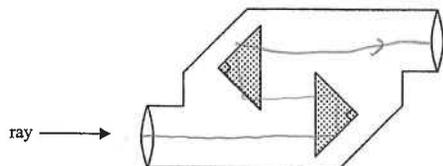
The Figure above shows the structure of part of a pair of binoculars, which consists of two triangular prisms.
