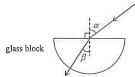
Figure 1 show a set-up used to study the relationship between the angle of incidence  $\alpha$  and the angle of refraction  $\beta$  of a ray of light travelling from air into a semi-circular glass block. Figure 2 shows a graph of  $\sin \alpha$  against  $\sin \beta$ .
