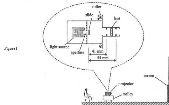
Peter designs a simple slide projector (see Figure 1). A slide is placed in front of a bright light source. A sharp image of the slide formed by a lens is projected onto a screen. The focal length of the lens is 40 mm and the distance between the slide and the lens can be adjusted within the range of 41 to 55 mm.
