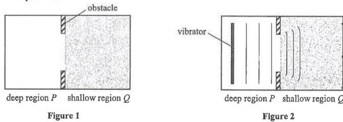
Figure 1 shows a ripple tank with a deep region  $P$  and a shallow region  $Q$ .
