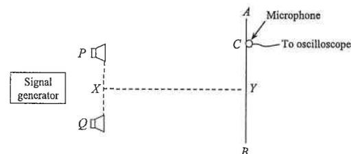
(a) Initially only  $P$  is connected to the signal generator and sound is emitted. A microphone connected to an oscilloscope is placed at point  $C$ . The below figure shows the trace on the oscilloscope. The speed of sound in air is  $325 \text{ m s}^{-1}$ . Find the frequency and wavelength of the sound. (5 marks)
