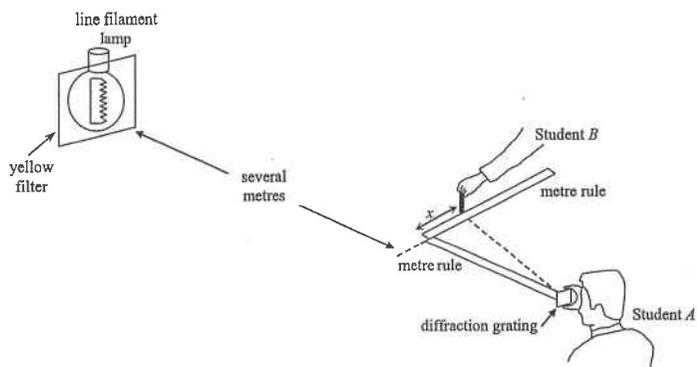
Student A views a line filament lamp with a yellow filter through a diffraction grating with its lines parallel to the filament as shown. The grating is held at one end of a metre rule which is directed towards the lamp. At the other end of the metre rule, a second rule is placed at right angles to the first rule. The diffraction grating has  $6.0 \times 10^5$  lines per metre.
