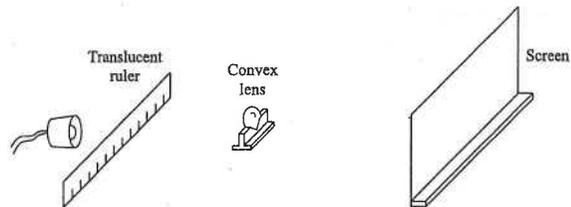
The figure shown above is a simple experimental set-up to study the image formed by a convex lens. The translucent ruler is an illuminated object, the position of which remains unchanged throughout the experiment. The position of the lens is adjusted so that a sharp image of the ruler is formed on the screen.
