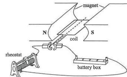
The figure shows a simple motor. Which of the following changes would increase the turning effect of the coil ?
