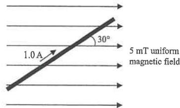
The figure shows a current of 1.0 A flowing in a metal rod of length 0.5 m. The rod is placed inside a region with a uniform magnetic field of strength 5 mT. What is the direction and the magnitude of magnetic force acting on the rod?
