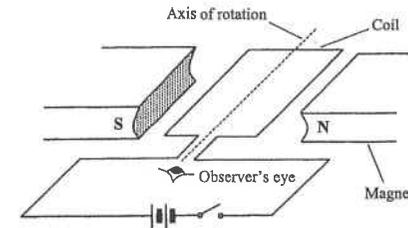
A rectangular coil can rotate in a magnetic field as shown in the above figure. Initially the coil lies horizontally. The switch is now closed.
