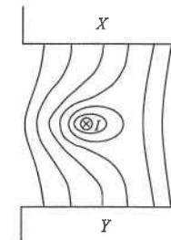
A straight wire carrying current  $I$  pointing into the paper is placed in a magnetic field between pole pieces  $X$  and  $Y$ . The figure shows the resultant field line pattern. What is the polarity of pole piece  $X$  and in what direction is the magnetic force acting on the wire? Ignore the effect of the Earth's magnetic field.
