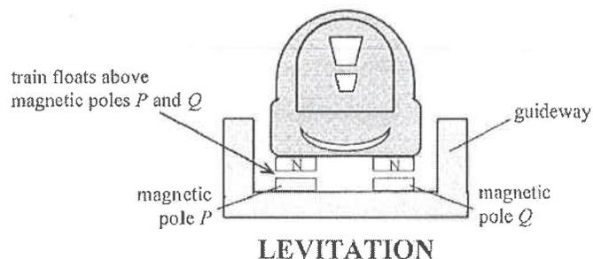
Two sets of magnetic fields are set up for different functions. One is to make the train float a few centimetres above magnetic poles *P* and *Q* as shown while the other is a propulsion system run by an alternating current for moving the train car along the guideway by magnetic attraction and repulsion. This floating design enables a smooth movement of the train. Even when the train travels up to 600 km per hour, passengers inside experience less vibration than travelling on traditional trains.
