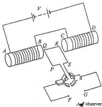
The figure above shows a simple experimental set-up to study the motion of a motor. *AB* and *CD* are solenoids connected to a battery *V*. *F* and *G* are connected to an external voltage supply. Its variation with time is shown in the following figure.
