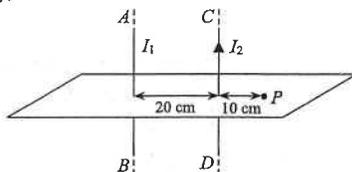
In the above figure,  $AB$  and  $CD$  are two parallel long wires with separation 20 cm carrying currents  $I_1$  and  $I_2$  respectively. The resultant magnetic field at the point  $P$  10 cm from wire  $CD$  is zero. If  $I_2$  is equal to 0.6 A, determine the magnitude and direction of the current  $I_1$  in the wire  $AB$ .
