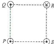
Four long straight wires perpendicular to the plane of the paper are placed at the four corners of a square  $PQRS$  as shown in the figure. Same current  $I$  flows in the wires at  $P$ ,  $Q$  and  $S$  directed into the paper while the current flowing along the wire at  $R$  is in the opposite direction. If the wire at  $P$  experiences no net magnetic force, find the current flowing in the wire at  $R$ .
