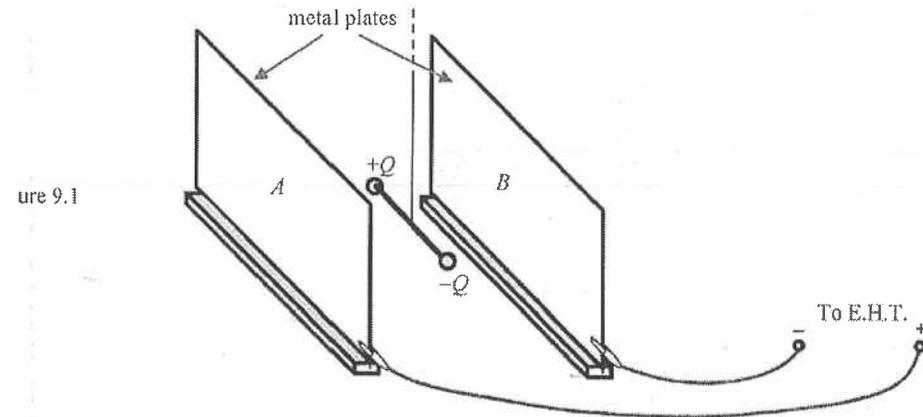
The rod is parallel to the metal plates when the E.H.T. is off. After the E.H.T. is switched on, an electric field is set up between the plates and the rod is twisted by an angle of  $20^\circ$  as shown in Figure 9.2.
