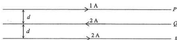
For two long, parallel, straight wires placed a distance  $d$  apart and each carrying a current of 1 A, the magnetic force per unit length is  $F$ . What is the resultant magnetic force per unit length acting on the wire  $R$  shown in the above figure?
