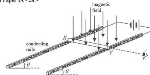
A copper rod  $XY$  is placed on a pair of smooth inclined conducting rails which are located in a magnetic field applied vertically downward. The rails make an angle  $\theta$  to the horizontal and a battery is connected to the rails as shown above. Which diagram shown below represents the magnetic force  $F_B$  acting on the rod when viewed from end  $Y$ ?
