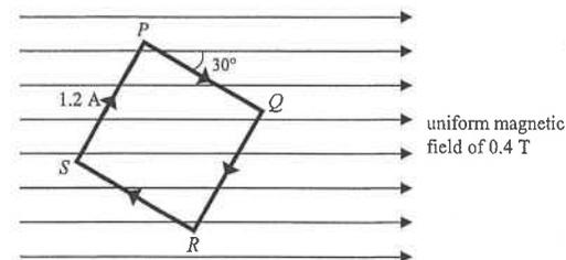
A square coil  $PQRS$ , each side has a length of 0.15 m is placed in a uniform magnetic field of 0.4 T as shown in the figure. The number of turns in the coil is 20 and the current in the coil is 1.2 A. The magnetic field is parallel to the plane of the coil. The side  $PQ$  makes an angle of  $30^\circ$  with the magnetic field. Find the magnetic force acting on the side  $PQ$  of the coil.
