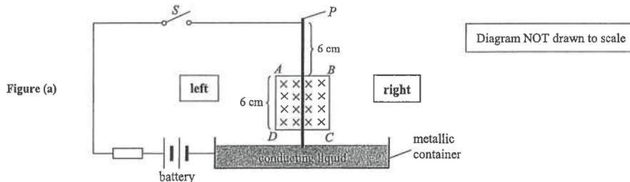
17. A uniform magnetic field pointing into the paper is applied over the region  $ABCD$  containing part of the rod. When switch  $S$  is closed, the rod 'kicks' out and leaves the liquid surface.
