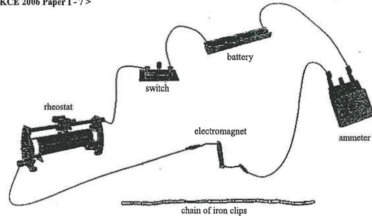
In a physics lesson, you are asked by the teacher to investigate the relationship between the strength of an electromagnet and the number of turns of its coil by using the apparatus shown in the above Figure. Describe the procedure for the experiment you should conduct. State clearly how you can measure the strength of the electromagnet. (5 marks)
