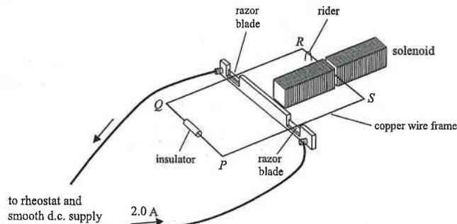
When a current of 2.0 A flows in the arm RS of the current balance, and the same current flows in the two solenoids in the same direction (not shown in the figure), placing a rider of mass 72 mg on the arm RS can restore the balance.
