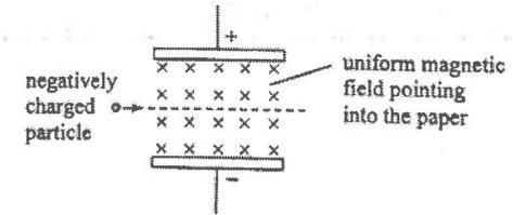
A negatively charged particle goes undeflected through a region in which a uniform electric field and a uniform magnetic field are set up as shown. The electric field is set up by the potential difference across the two parallel metal plates. Which of the following changes may cause the charged particle to deflect downward? Neglect the effects of gravity.
