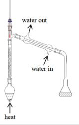
mark for the sketch: including the pear-shaped flask, fractionating column (with something inside), thermometer, condenser, adapter and a container (such as conical flask, beaker) (Accept: space with thermometer inserted/close system)
